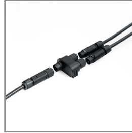
Ordering Code: AUN-CON-0010-00 IP68 Water Tight Connecting Device with Distribution block, 3 pole, 1 input, 2 outputs, Cable Diameter 5.0 – 9.5mm.
